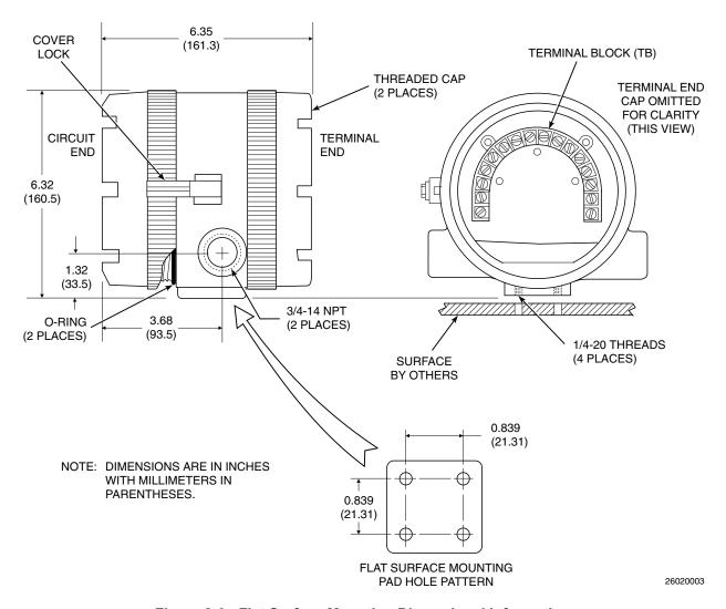
Figure 2-6. Flat Surface Mounting Dimensional Information
